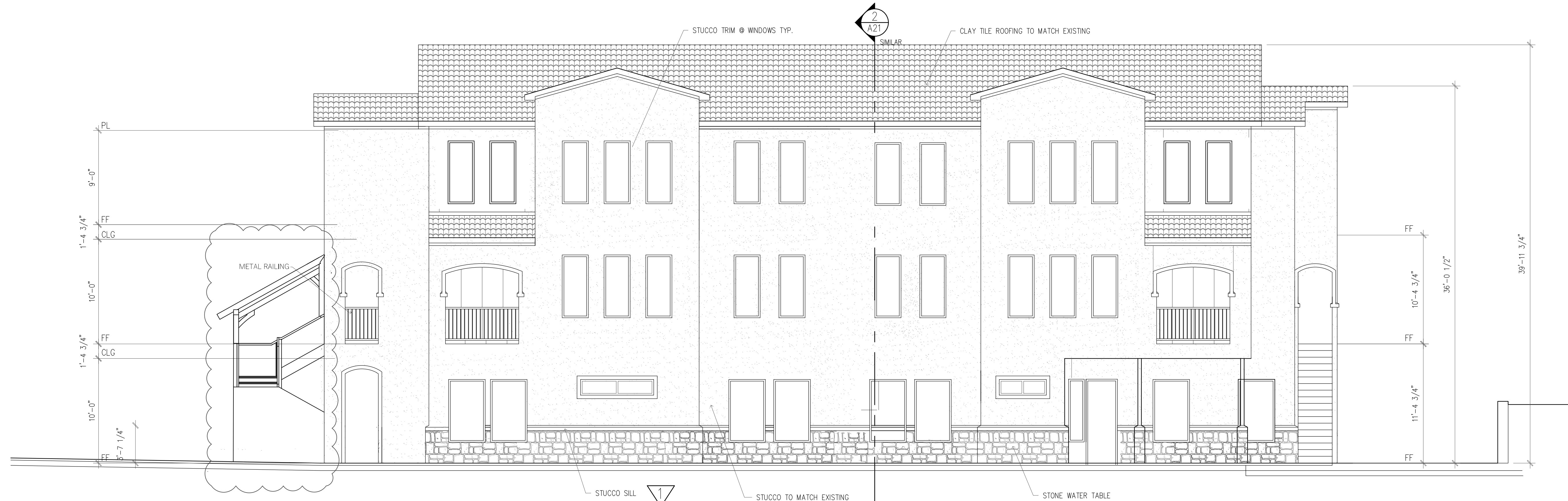
NORTH ELEVATION 100% MASONRY 10% STONE 90% STUCCO
